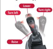
To prevent malfunctions, the operator must press the vessel lock release switch to raise or lower the vessel.
