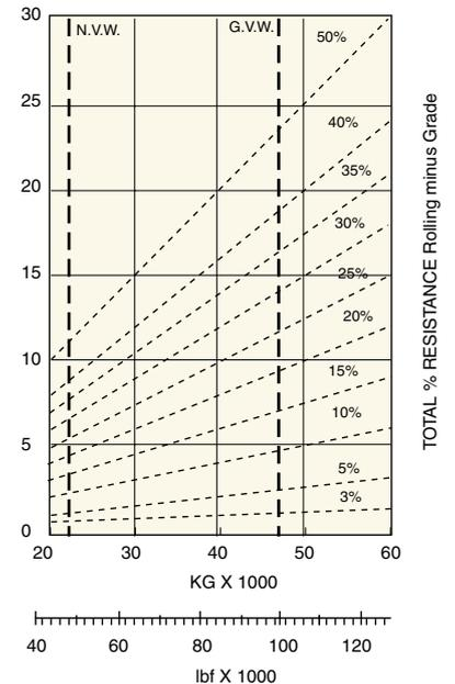
Instructions: From intersection of vehicle weight with percentage resistance line read across to determine maximum gear attainability, and then downwards for speed.
