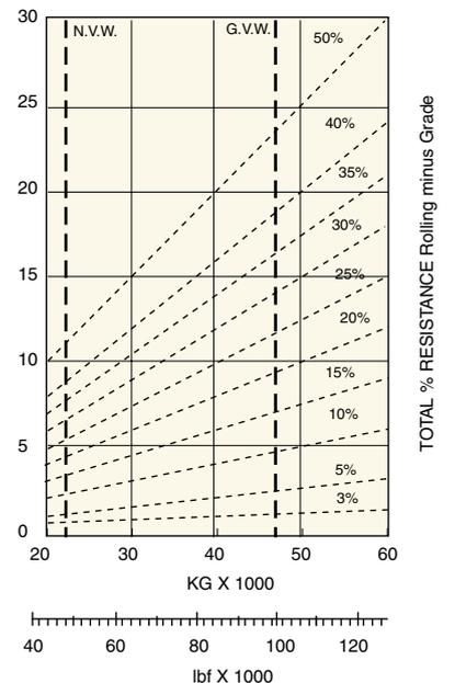
Instructions: From intersection of vehicle weight with percentage resistance line read across to determine maximum gear attainable, and then downwards for speed.
