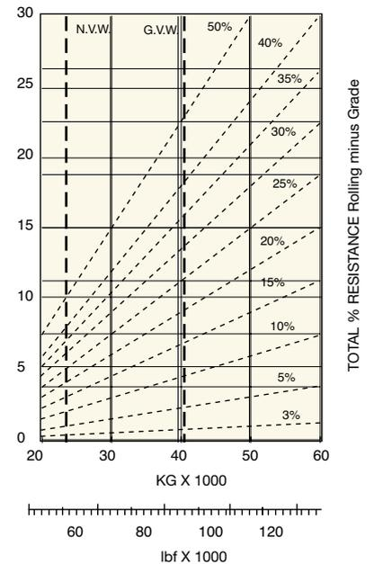
Instructions: From intersection of vehicle weight with percentage resistance line read across to determine maximum gear attainable, and then downwards for vehicle speed.
