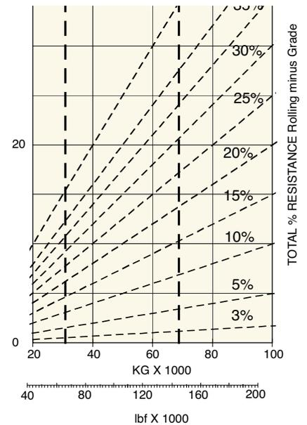
Instructions: From intersection of vehicle weight with percentage resistance line read across to determine maximum gear attainable, and then downwards for speed.
