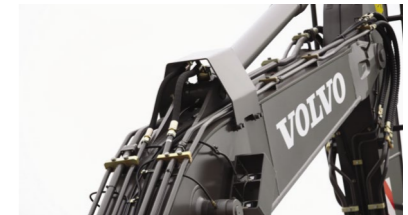
Factory high lift boom and arm with heavy duty forestry guarding, integrated piping, hydraulic cylinder and work light guarding.
