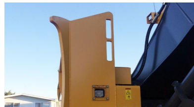
Heavy duty right-side body deflector rail and reinforced right corner guard post. With spacious lockable tool storage.
