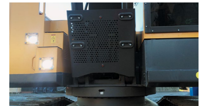
Boom cylinder guard. Optical boom foot riser increases boom and arm reach and overall machine stability.
