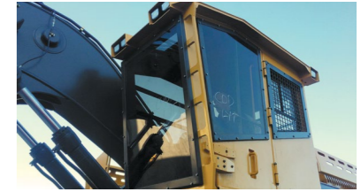
Volvo Forestry Care Cab with standard 400 mm cab riser and full forestry guarding meets global safety standards. Front window is 32 mm safety glass.
