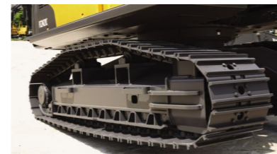
Heavy duty full length track rock guards. Dual mounted bottom rollers on top. Reinforced idlers with derail guards.
