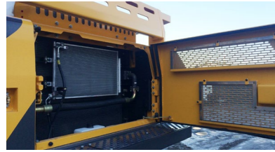
Reinforced side doors with heavy duty screens protect coolers and pumps while providing maximum air flow.
